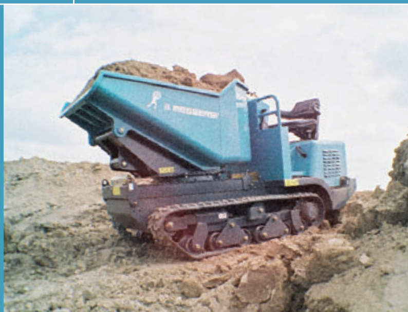
180° TCH-1500/BT swivelling skip during working phases / TCH-1500/BT mit 180° Drehmulde in Arbeitsphase / Бункер модели TCH-1500/BT вращается на 180°.
