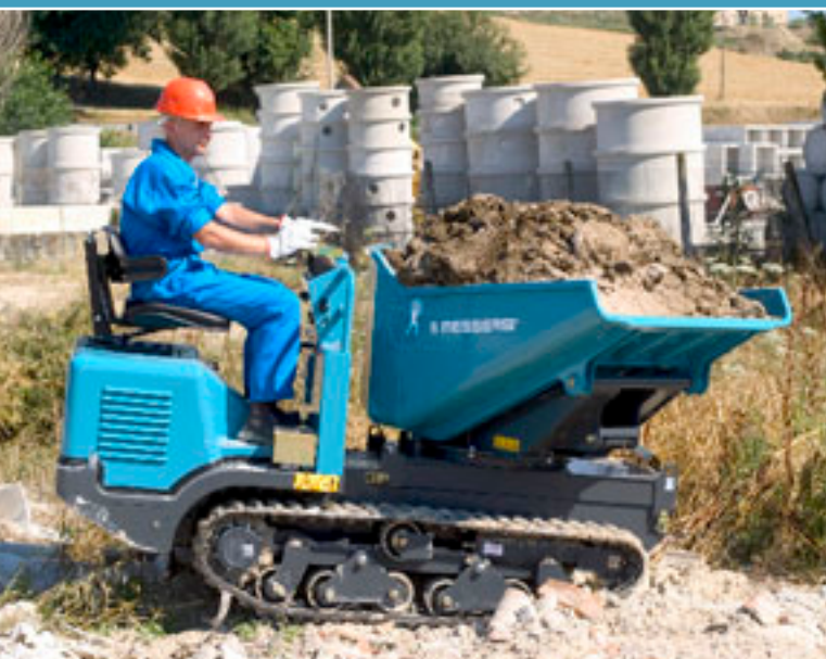
180° TCH-1500/BT swivelling skip during working phases / TCH-1500/BT mit 180° Drehmulde in Arbeitsphase / Бункер модели TCH-1500/BT вращается на 180°.
