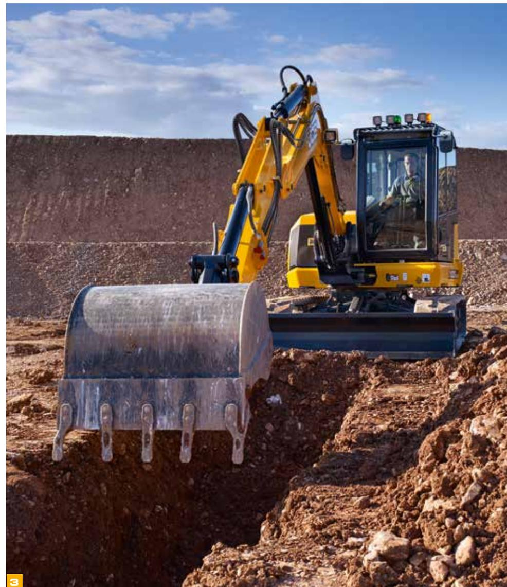
3 The fully compliant ROPS and TOPS\* cab has excellent front visibility courtesy of a 70/30 front screen split. It also provides a clear view of the front right track for easy, safe trench digging and manoeuvring. Overall, we have improved overhead visibility from the cab making truck loading easier and safer.
